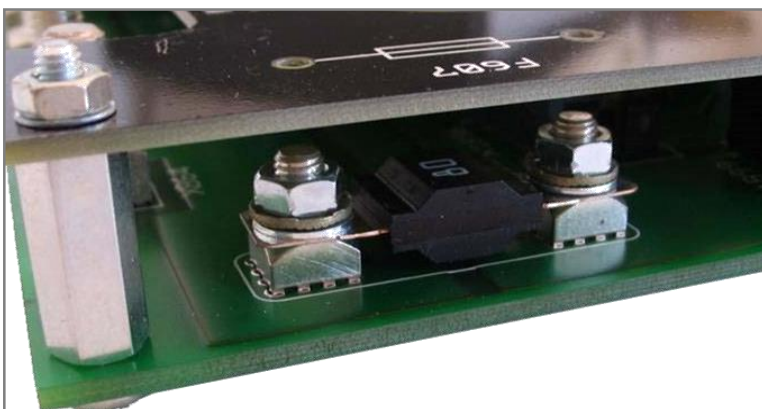
Mounting of laminated fuses
