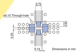
Line width be designed to match  $50\Omega$  characteristic impedance depending on PCB material and thickness.
