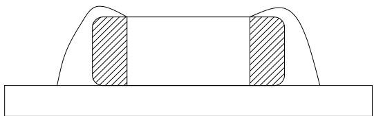
Too Much Solder large stress may cause cracks
